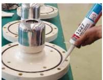
High Voltage Switch Flange Sealing
